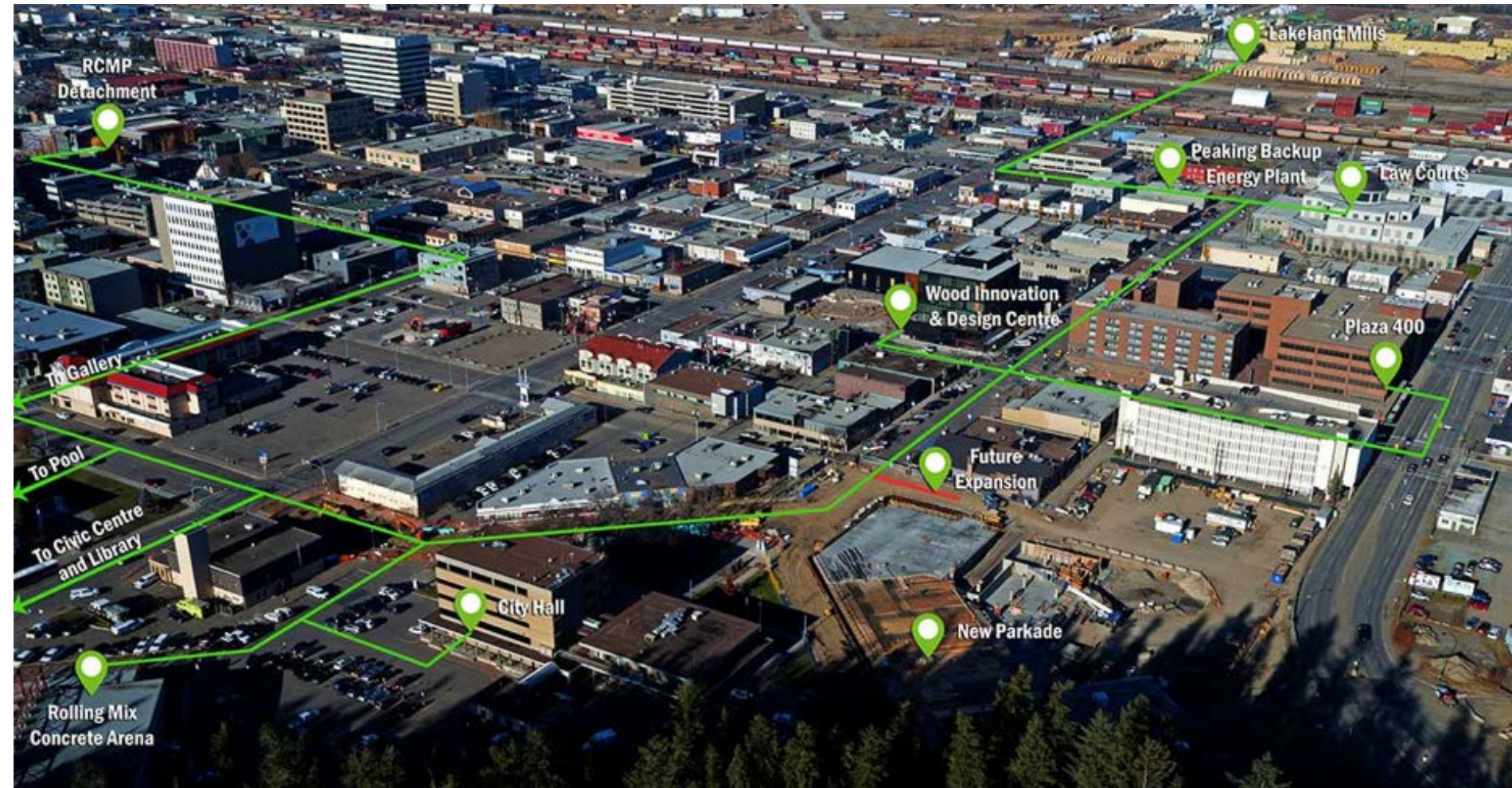
Figure 6 – Map of City of Prince George Downtown Renewable Energy System, indicating most of the distribution piping network and connected buildings.
