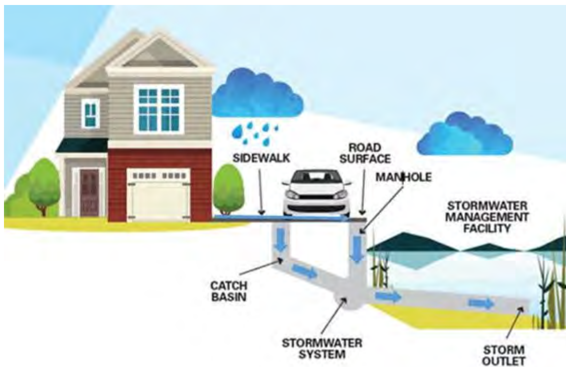
Figure 2: Typical Municipal Stormwater System
