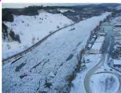
TYPICAL JUXTAPOSED ICE COVER, NOTE THE WELL DEFINED ICE FLOES SITTING FLAT ON WATER SURFACE.
