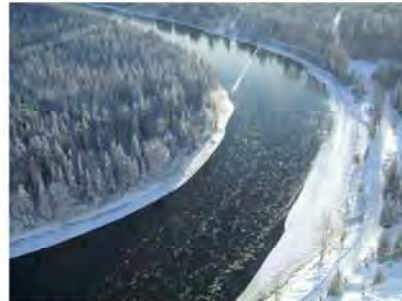
VERY LIGHT ICE RUN UPSTREAM OF PRINCE GEORGE. MOST OF ICE WILL BE IN SUSPENSION AS THIS IS THE START OF THE SUSPENDED ICE FLOATING TO THE SURFACE AND FIRST FORMING INTO SURFACE ICE FLOES.
