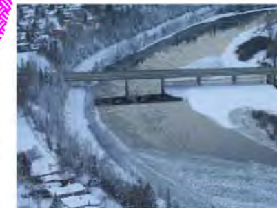
MEDIUM TO HEAVY ICE RUN UPSTREAM OF ICE FRONT. IN THIS SITUATION MOST OF THE FRAZIL WILL BE ON THE SURFACE, WITHIN THE ICE FLOES (PANS). THERE WILL ONLY BE A SMALL AMOUNT OF SUSPENDED FRAZIL ICE.
