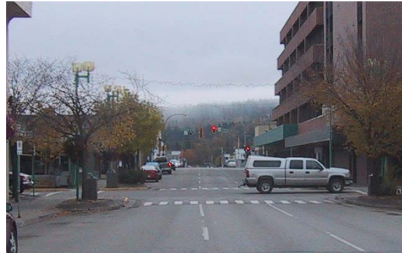
4 th Avenue and George Street Street furniture and landscaping on corner bulges can block view of waiting pedestrians.
